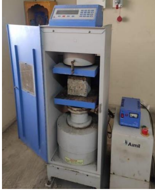
Fig. 4. COMPRESSION TESTING MACHINE (CTM)
