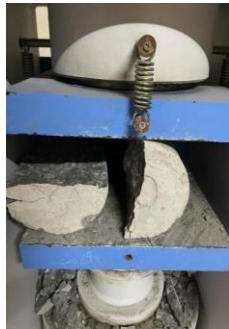
Fig. 5. SPLIT TENSILE TESTING
