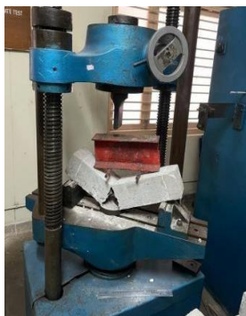
Fig. 6. FLEXURAL STRENGTH TESTING
